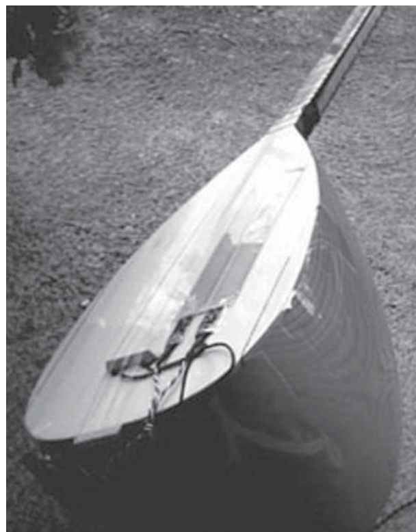
Figure 2. eSaz body displaying sensors within reach of the plucking hand and on the bottom of the neck.
