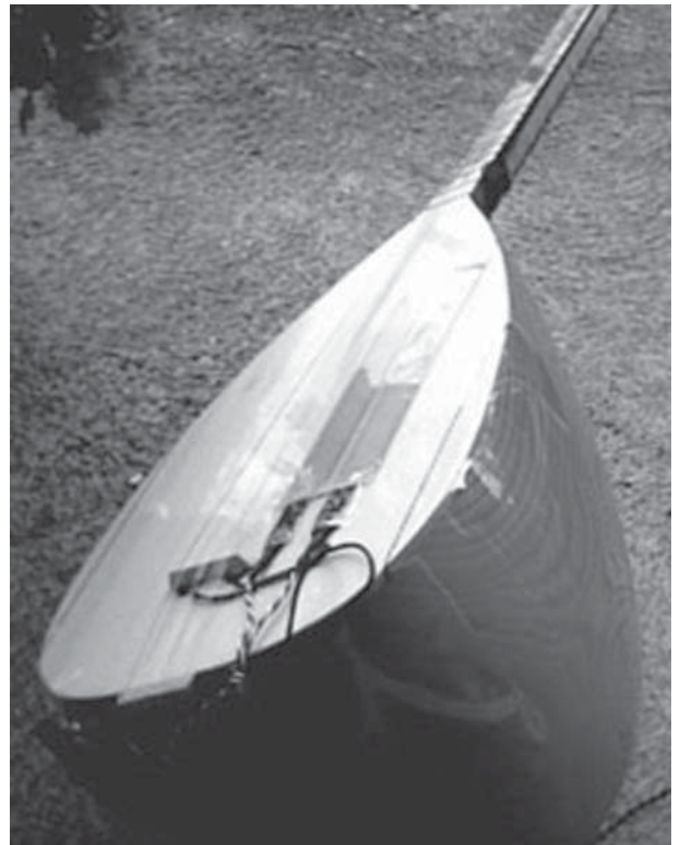
Figure 2. eSaz body displaying sensors within reach of the plucking hand and on the bottom of the neck.
